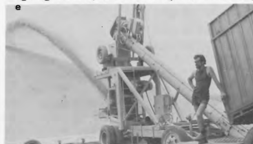
Fig. 8. Various views and uses of the grain auger (screw conveyor): (a) rear view of extractor auger; (b) extractor auger used to outload grain from silo and elevating auger to load it into rail wagons; (c) extractor auger as used for outloading grain from a shed; (d) extractor and elevating augers filling rail wagon from temporary (portable) road dump pit; (e) extractor auger used for feeding grain to belt slinger for pad storage filling.
