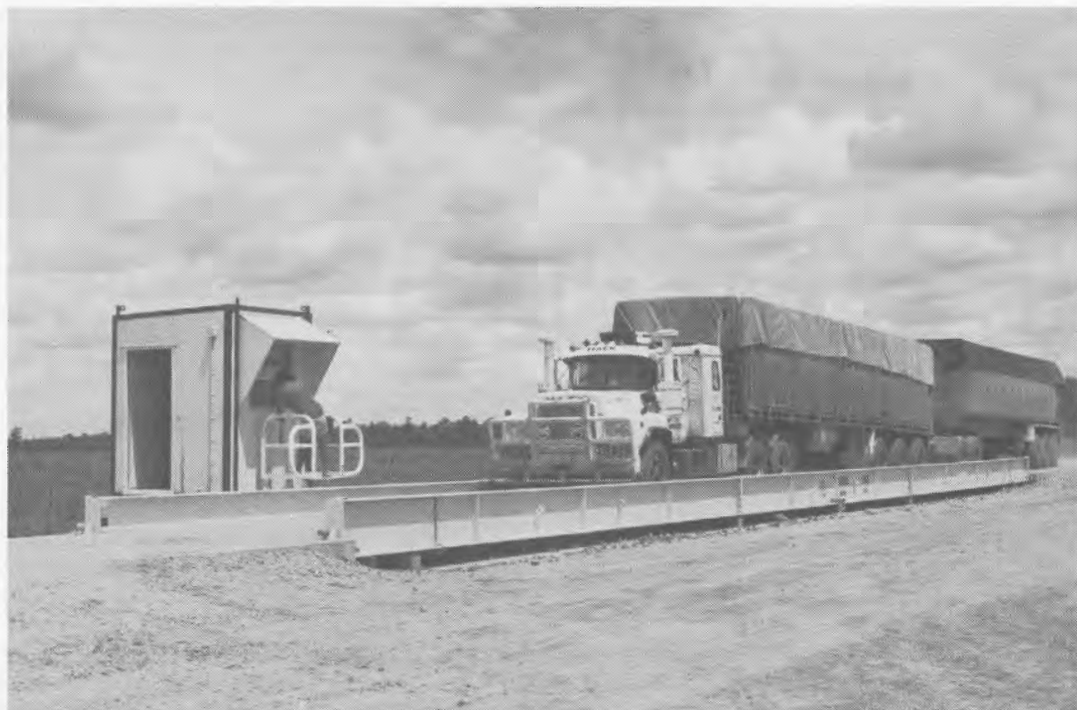
Fig. 24. A pitless weighbridge, 33 m long and of 100 tonnes capacity.
