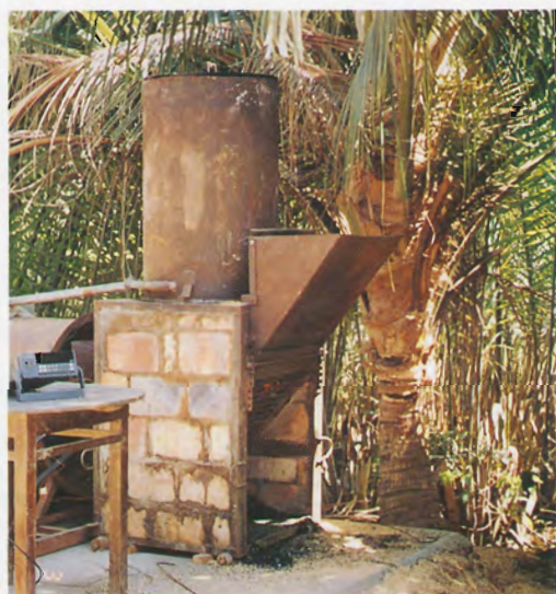
Figure 3. Inclined grate furnace with cyclonic ash separator.
