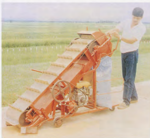
Figure 1. The pavement grain collector designed by IRRI.
