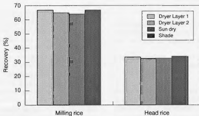
Figure 9. Milling quality of paddy dried using the SRR-1 dryer (25–30 August 1995) compared with sun and shade-dried paddy.
