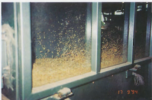
Figure 7. Prototype 1 t/hour fluidised-bed paddy dryer.
