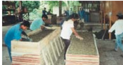
Figure 1. Small-scale wood-wool cement board plant in the Philippines showing the process of forming boards by hand
