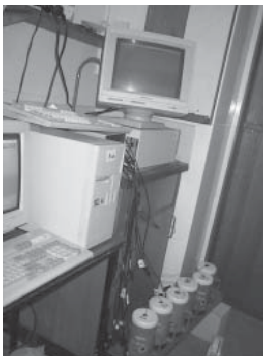
Plate 3. Hydration temperature-logging apparatus in controlled climate room
