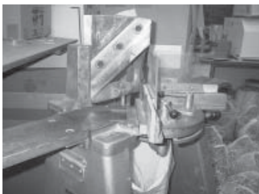
Plate 2. Guillotine used to slice wood flakes with catcher bag attached
