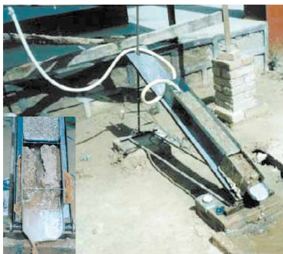
Figure 1. Mini-flume for soil antiscourability test.
