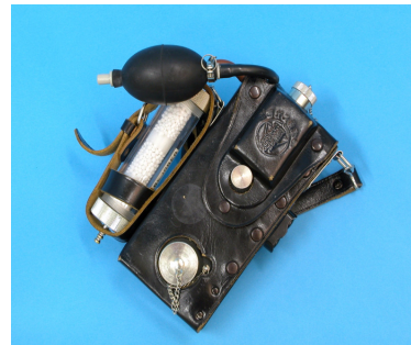
An interferometer used to measure methyl bromide at fumigation concentrations.
