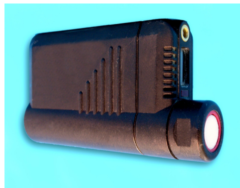
An electronic instrument that measures phosphine at health and safety levels.
