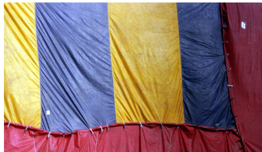
Sheets joined by rolling, held together by spring clips
