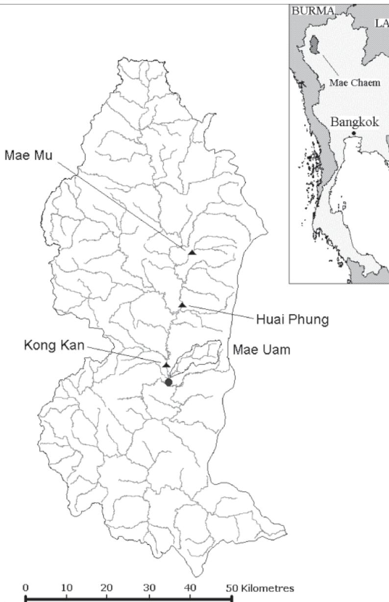
**Figure 6.4** Location of discharge gauges and the ungauged Mae Uam sub-catchment used to test the regionalisation procedure and model response to forest-cover changes. The large dot gives the location of Mae Chaem city. Source: Merritt et al. (2004).
