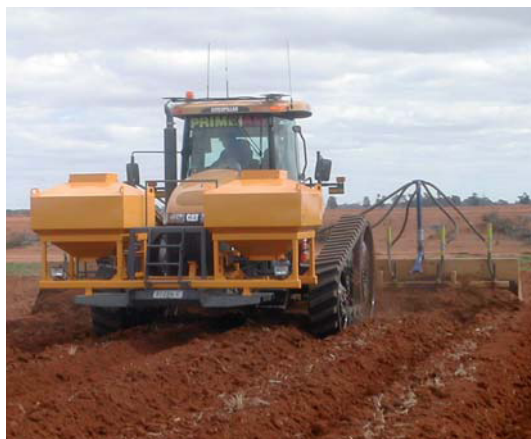
Figure 7. Fertiliser being applied during bed shaping (in a one-pass operation) in construction of raised beds.
