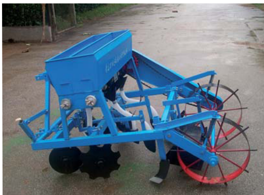
Figure 3. Left – The planter for raised bed planting; Right – Making bed, applying fertiliser and sowing wheat at same time.
