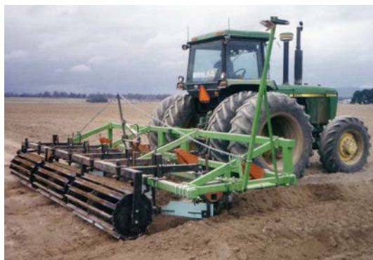
Figure 5. A bed-former used in Southern Australia.
