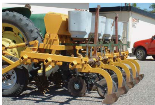
Figure 2. Left – Multi-crop/multi-use implement configured for reshaping permanent beds and applying basal fertiliser; Right – The same implement configured for bed reshaping, fertilising and maize planting.
