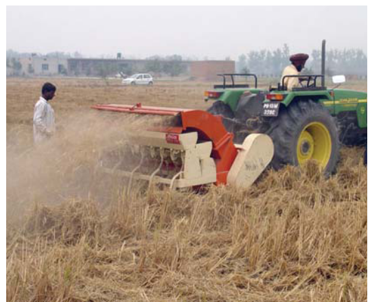
Figure 5a and 5b. The Happy Seeder combines stubble mulching and seed drilling functions into one machine (J. Blackwell and H.S. Sidhu).
