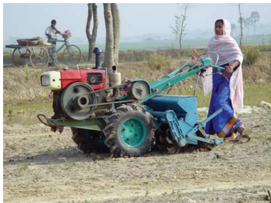
Figure 3. Chinese hand tractor with power operated tiller/ seeder (POTS) and 48-tine tiller, seeder and compactor attached (C.A. Meisner).
