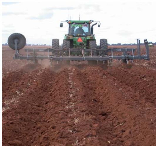
Figure 9. High powered tractor using a toolbar equipped with furrow sweeps to create furrows and beds.
