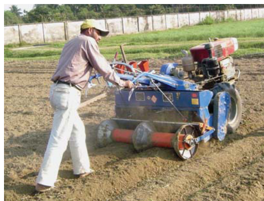
Figure 6. Bed former based on POTS with the Chinese hand tractor with square and cone shapers (C.A. Meisner).
