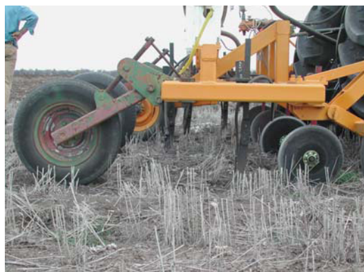
Figure 10. Modified anhydrous ammonia rig with coultter discs in front of gas knives (Hulugalle et al 2004b).
