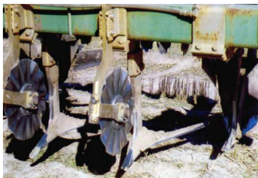
Figure 9. Machine used to renovate PRBs. Blades pass through the base of the PRBs level with the base of the furrows, causing zero soil inversion.
