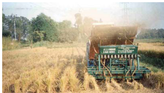
Figure 7a. Sowing wheat into rice stubble on beds with first prototype of the Happy Seeder at Ludhiana, October 2002 (John Blackwell).
