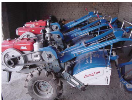
Figure 1. Chinese hand tractor with 18-tine tiller attached (C. Meisner).
