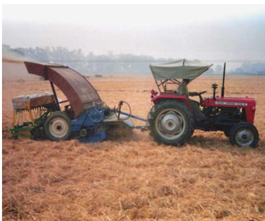
Figure 5a and 5b. The Happy Seeder combines stubble mulching and seed drilling functions into one machine (J. Blackwell and H.S. Sidhu).
