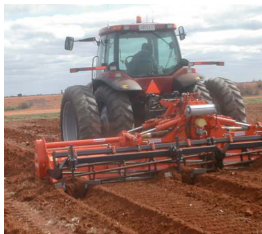
Figure 11. Level and smooth seeding surface being created on raised beds by use of a rotary hoe and rotary harrows.
