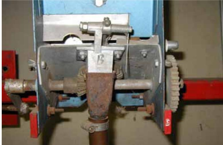
*Figure 180: the rear view of an inclined plate type seed meter*
