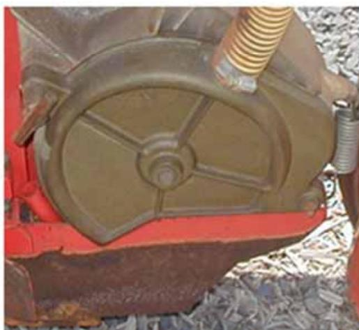
Side view of a vacuum disc seed meter
