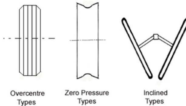
Figure 124: The three general types of press wheel
