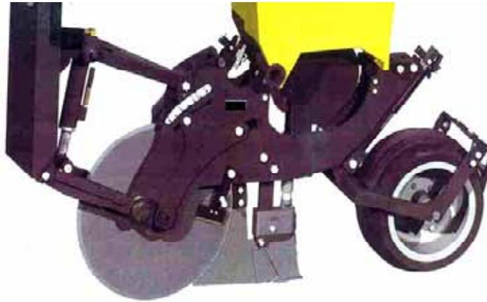
*Figure 61: A planter utilising a single aligned disc coulters type opener*
