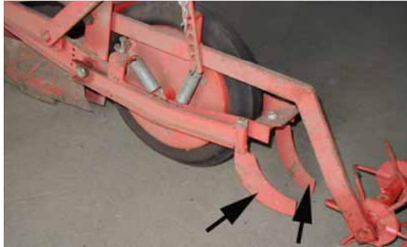
Figure 114: Opposed knife type covering devices
