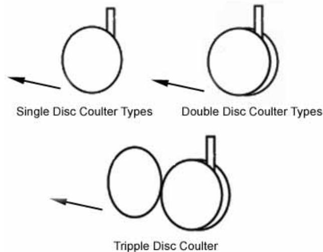
Figure 56: General types of disc coulters furrow openers
