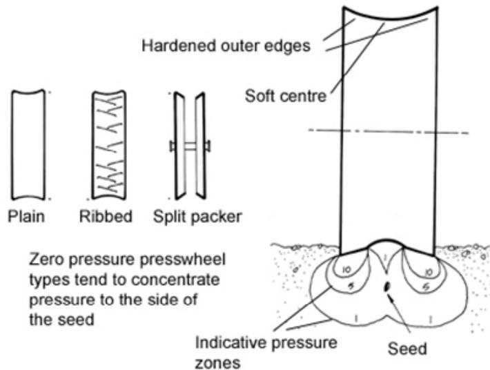
*Figure 127: Typical zero pressure press wheel profiles*
