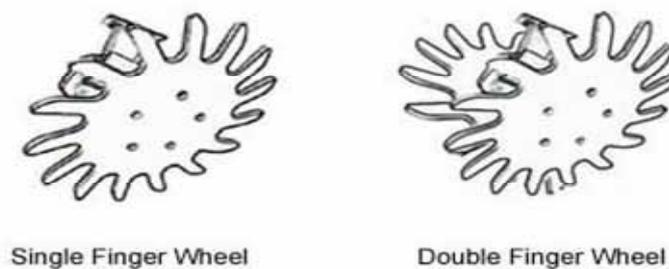
Figure 28: Typical single- and double- finger wheel configurations
