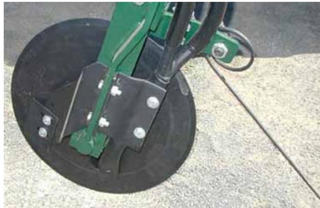
*Figure 120: A single finger type covering device*
