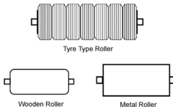
Figure 140: Some types of rollers used as non row specific seedbed firming devices
