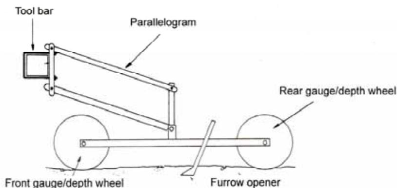
Figure 153: 'Twin' gauge wheel positions for parallelogram systems
