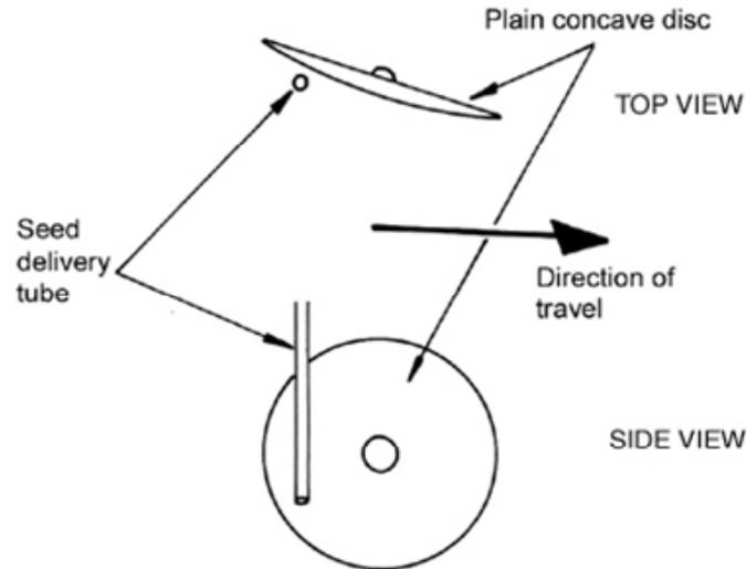
Figure 54: A concave disc type furrow opener
