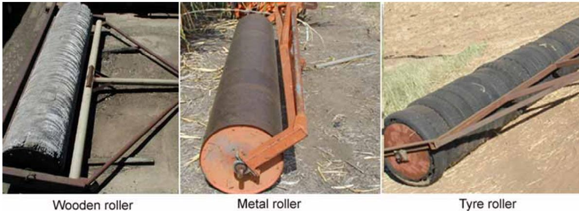
Figure 141: Examples of roller types
