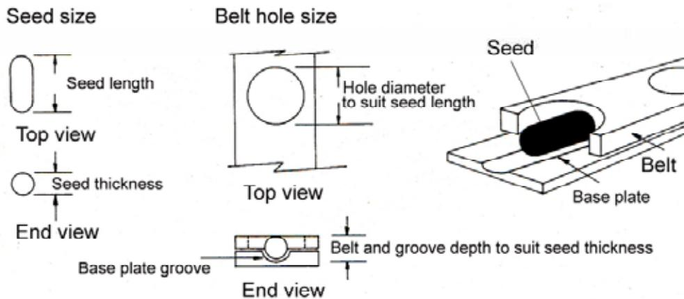
Figure 191: An example of the belt and base plate combination for a large cylindrical seed
