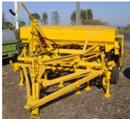
*Figure 11: A 14-row, trailed, tractor-powered drill planter*
