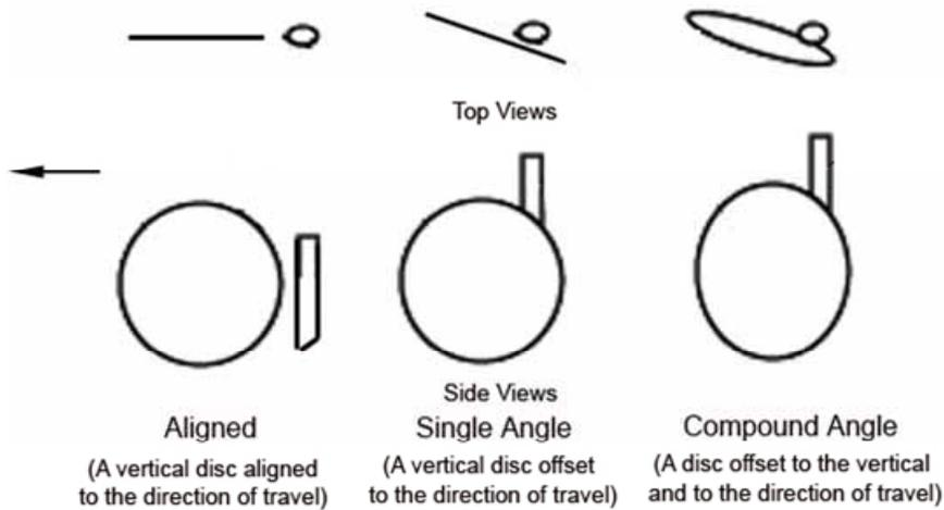
*Figure 57: Types of single disc coultter furrow openers*
