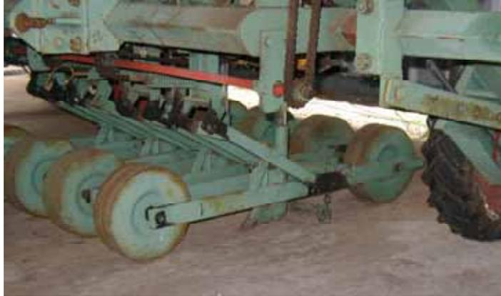
*Figure 162: A twin wheel type of the trailing arm system of depth control*
