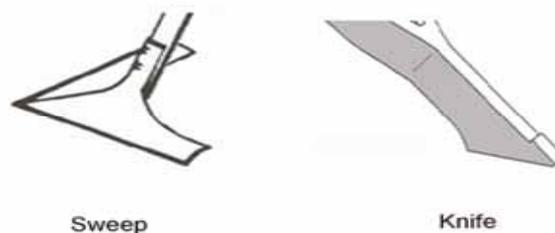
Figure 40: Typical tine type row preparation devices
