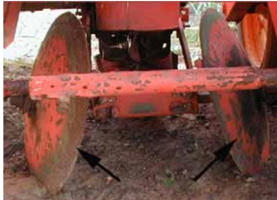
Figure 109: Rear view of a double concave disc type covering device
