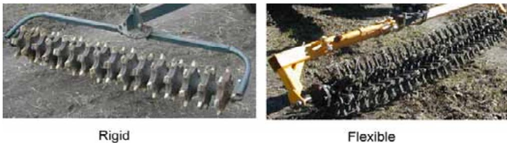
*Figure 144: Examples of rigid and flexible rotary harrows*
