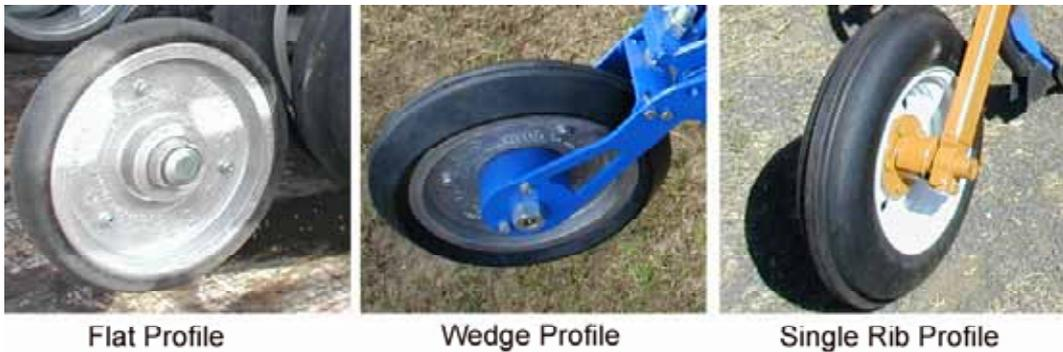
*Figure 126: Some types of over-centre press wheel profiles*
