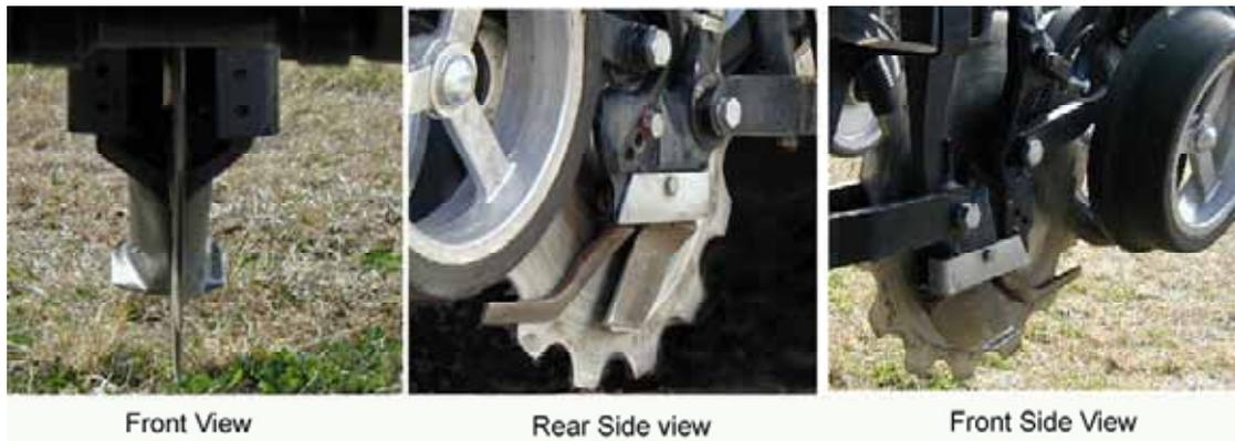
Figure 97: Front, rear and side views of the bioblade type furrow opener
