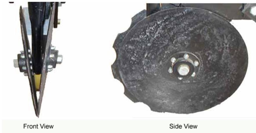
*Figure 76: A staggered twin inclined double disc coultter with a notched leading coultter*
