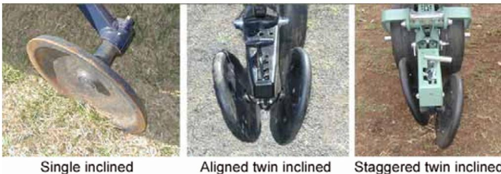
*Figure 131: Examples of Inclined press wheel types*
