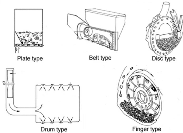
Figure 174: General types of precision seed metering devices
