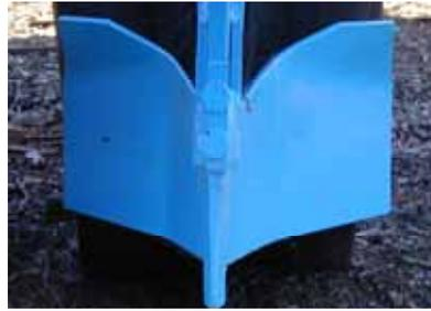
Figure 27: Example of a blade type row preparation device
