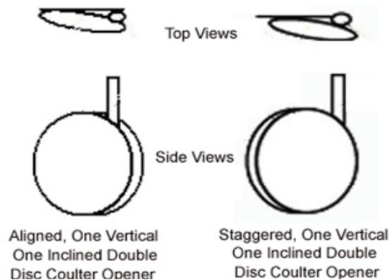
Figure 73: Design options within one-vertical one-inclined types of double disc opener
