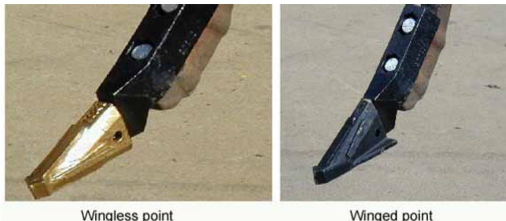
Figure 84: Winged and wingless versions of the same basic opener shape
