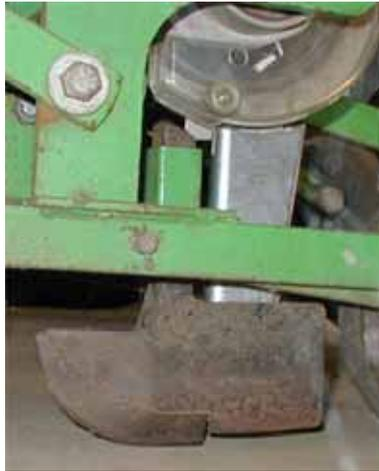
*Figure 53: Seed delivery via a short dropper tube*
