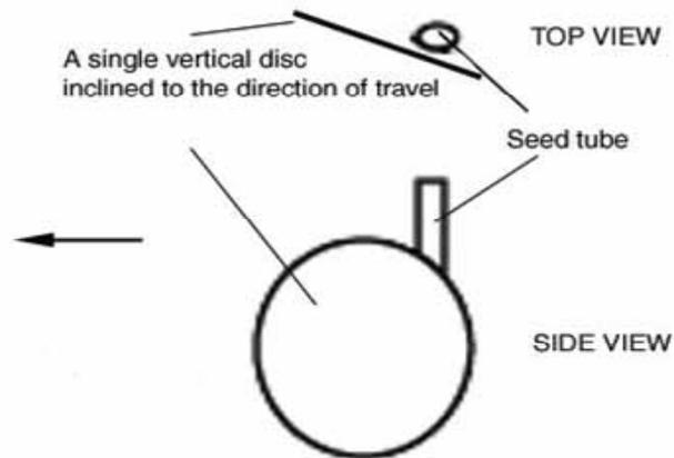
Figure 59: Single-angle single disc coulters type opener
