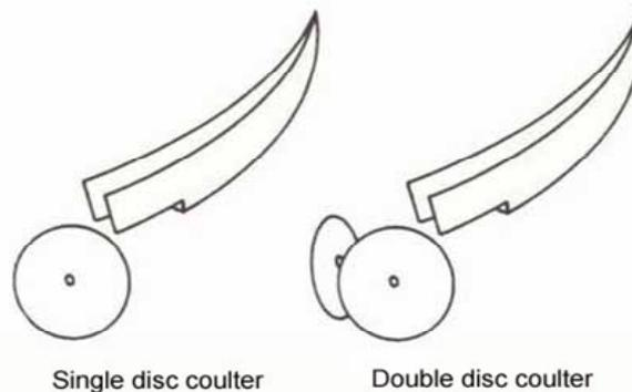
Figure 110: Single and double disc coulters type covering devices
