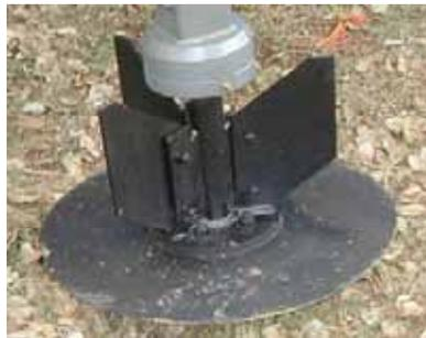
*Figure 45: An example of a horizontal disc type row preparation device*
