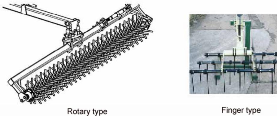
*Figure 143: Examples of 'rotary' and 'finger' type harrows*
