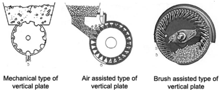
*Figure 182: General types of vertical plate meters*
