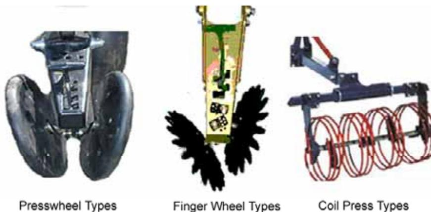
Figure 123: Types of seedbed firming devices
