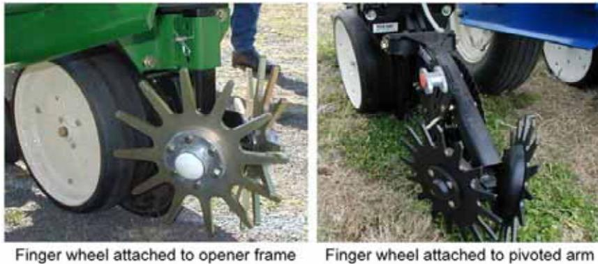
Figure 32: Spring steel finger wheel row preparation device
