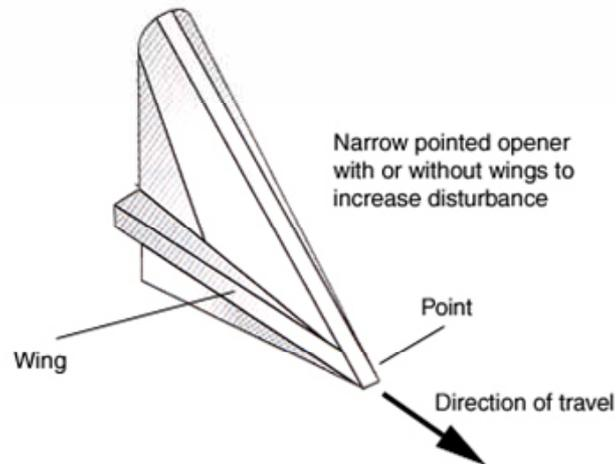
Figure 83: the general form of point type tine openers
