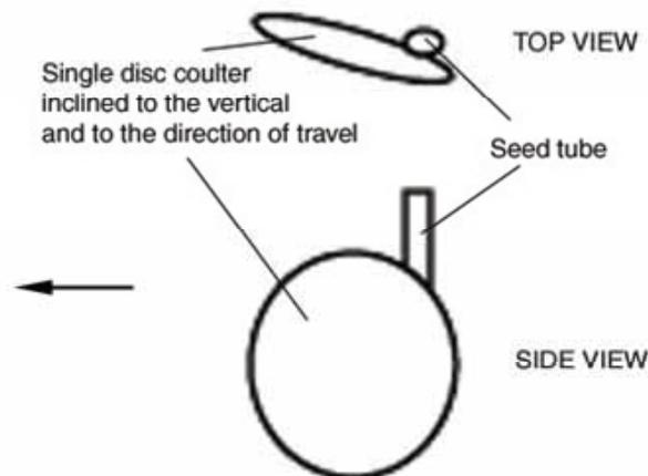
Figure 60: Compound-angle single disc coulters type opener
