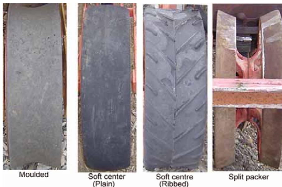
*Figure 128: Zero pressure press wheel types*
