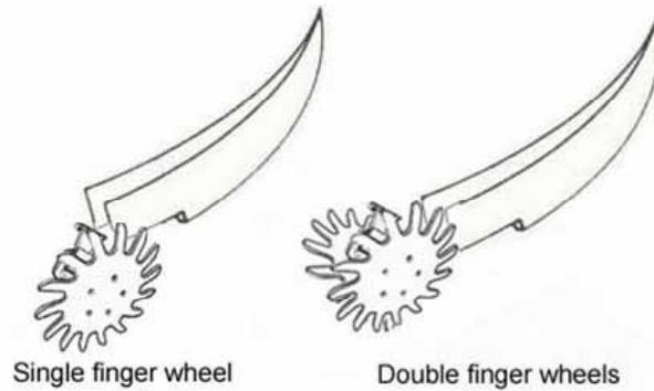
*Figure 121: Single and double finger wheel covering devices*
