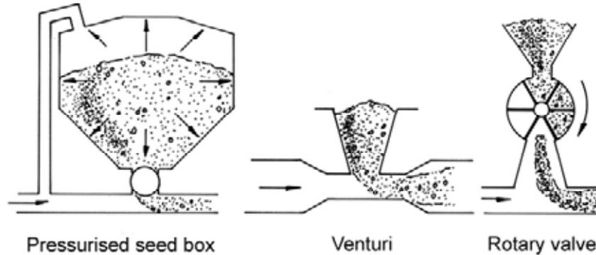
Figure 212: Common methods used to load the airstream
