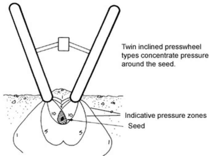
*Figure 130: Indicative pressure zones for inclined press wheels*
