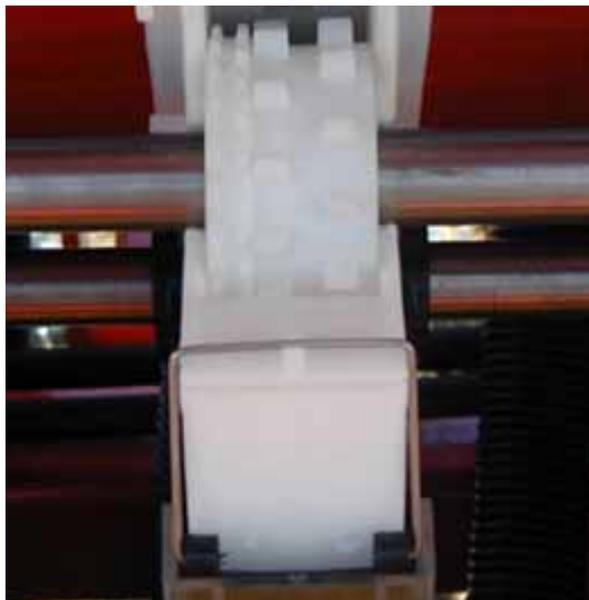
*Figure 170: The rear view of a peg or studded external force feed seed metering system*
