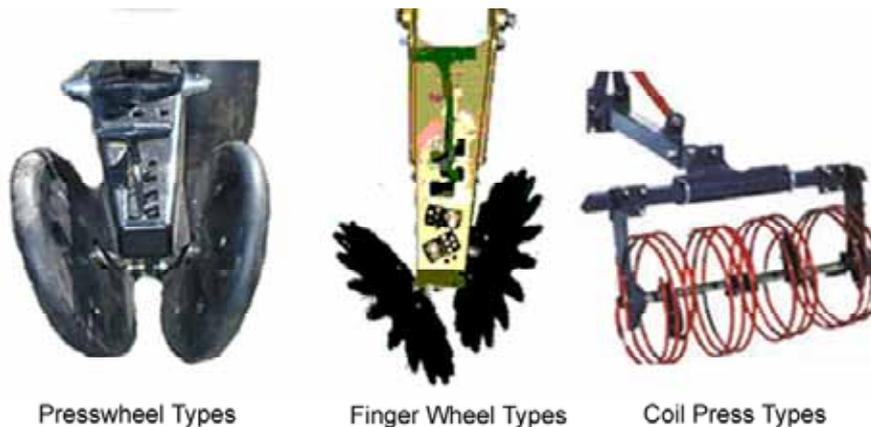
Figure 123: Types of seedbed firming devices
