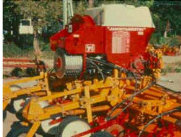
Figure 196: A rear side view of a pressurised drum precision seed metering unit
