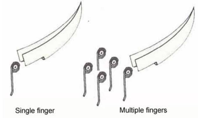
*Figure 119: Single or multiple finger type covering devices*
