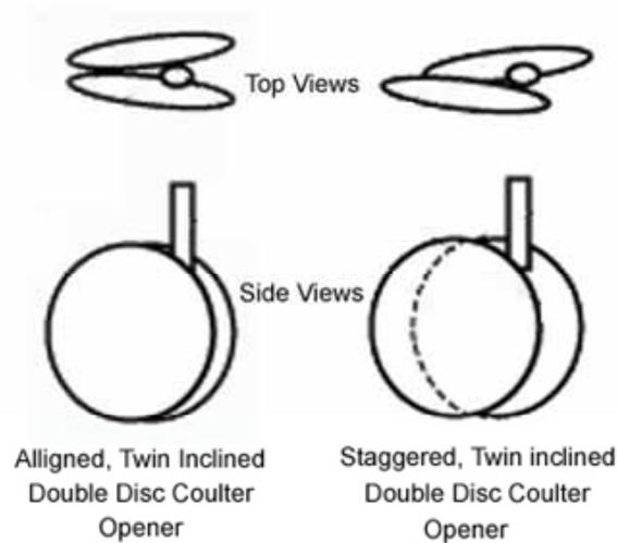
Figure 72: Design options within twin inclined types of double disc opener
