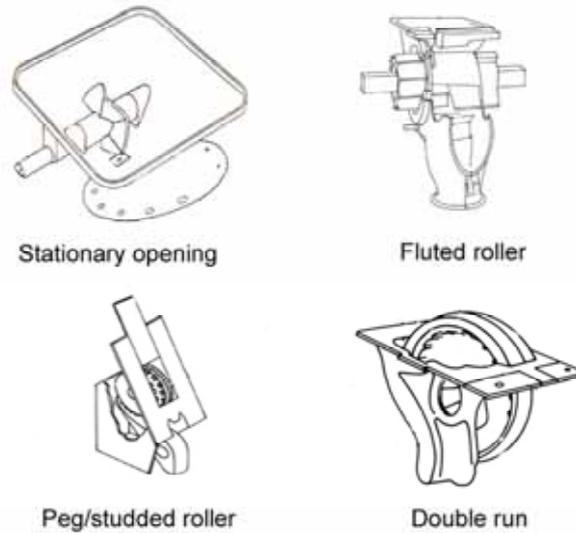
Figure 163: General types of mass flow seed metering devices
