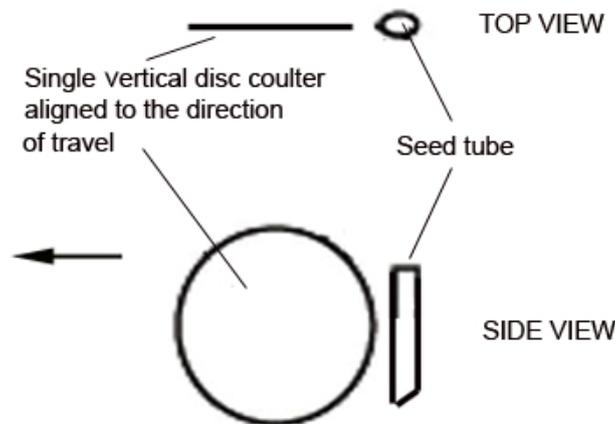
*Figure 58: Single, aligned disc coultter opener type*
