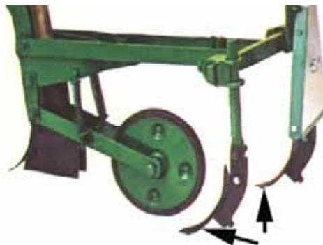
*Figure 118: Tine type covering devices fitted with reversible point type ground tool*
