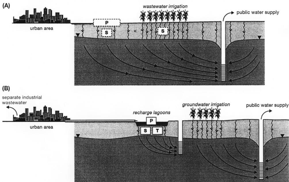
**Figure 8.** General schematic diagram of wastewater generation, treatment, reuse and infiltration to aquifers (from Foster et al. 2003). P, S and T denote primary, secondary and tertiary sewage treatments.
