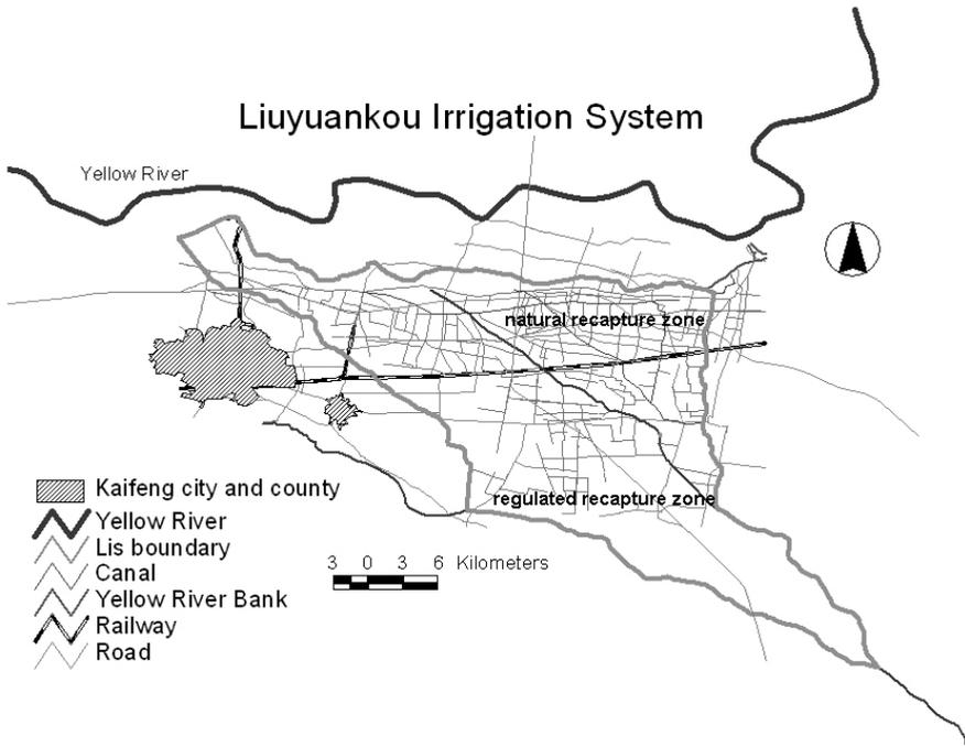
**Figure 2.** Layout of the Liuyankou Irrigation System (LIS). The rice area served by canals is north of the railway line, while the diversified cropping system supported by groundwater lies south of the line.
