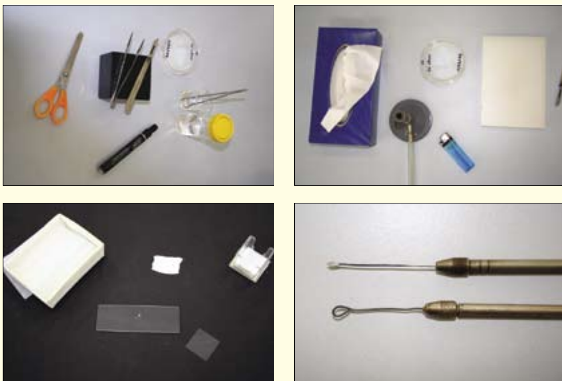
Figure 13.3 Essential instruments for isolation, subculturing, purification and identification of fungal and bacterial plant pathogens
