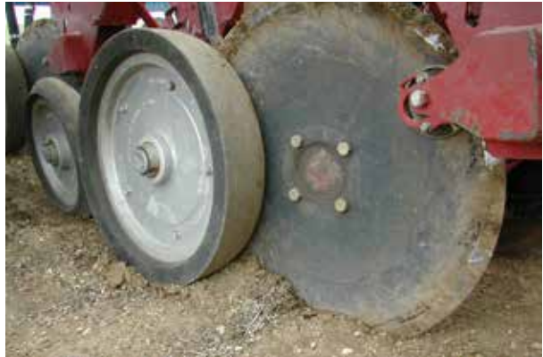
Figure 18. Examples of Australian seeding systems - a simple spring loaded tine (left), and a heavy duty single disc with gauge wheel (right).
