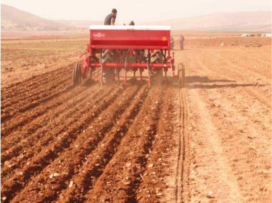
Figure 38: Sowing at high speed creates excessive 'soil throw' and variable seed depth. Note how the rows created by the front tines have been covered by the rear tines and the only furrows visible were created by the rear tines.
