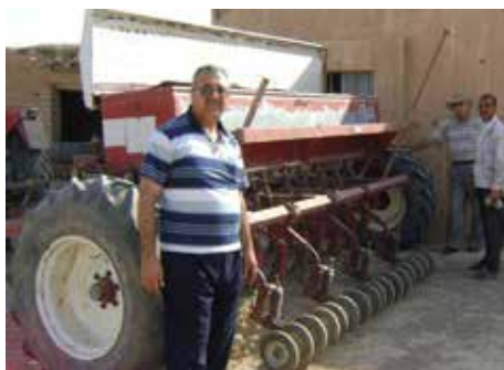
Figure 29. Mr. Ghazi Fathi from Mosul Iraq converted his Rama seeder to ZT and installed locally made press wheels.
