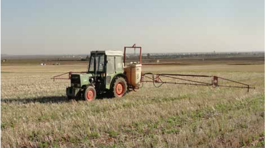
Figure 40. Most chemical sprays are applied with a boomsprayer which should be well maintained, calibrated and used in the appropriate way.
