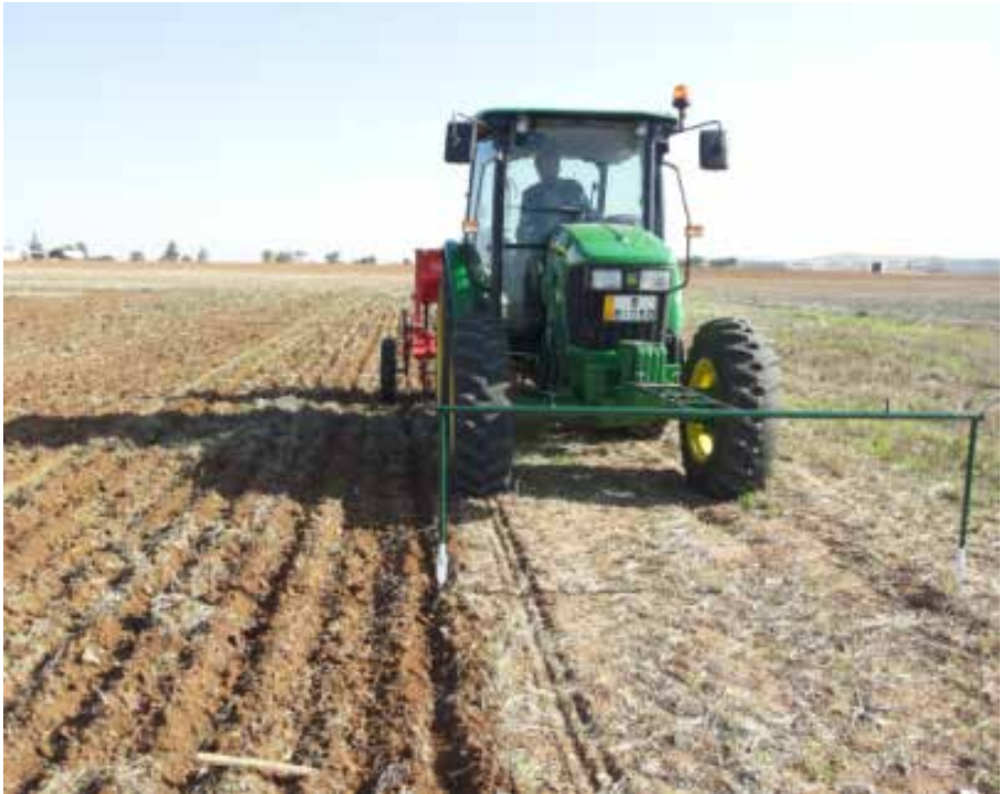
Figure 37: An example of a cheap guiding arm developed by ICARDA at the Mushaghar experimental station in Jordan, eliminates overlaps or gaps between sowing runs.
