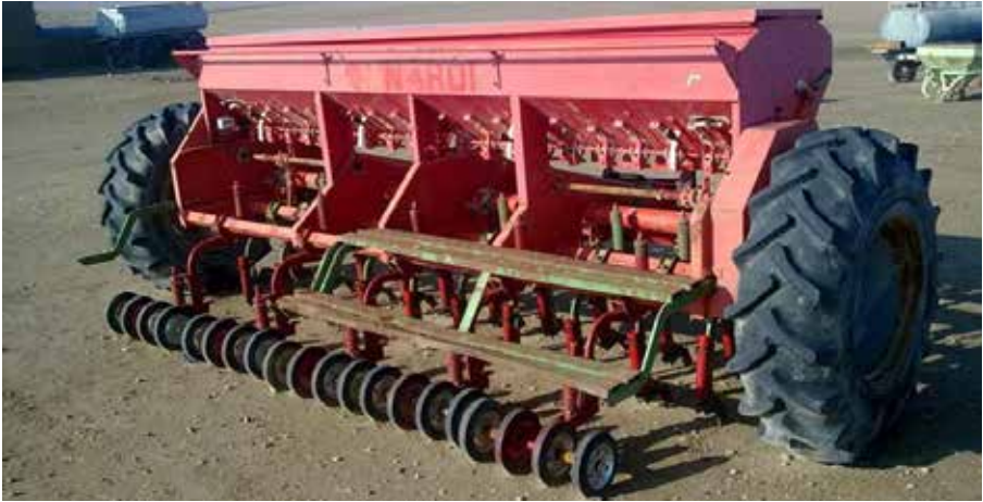
Figure 50. A Nardi seeder converted to ZT, including press wheels manufactured in Mosul Iraq.
