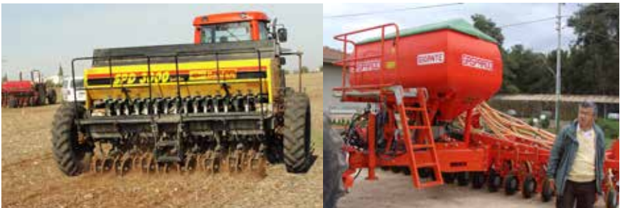
Figure 31. These Brazilian and Italian disc ZT seeders imported into the Middle East can perform well in suitably mechanized ZT systems, but are relatively complex, heavy and expensive for small farmers.
