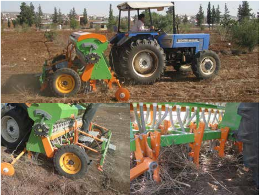
Figure 26. This Turkish made conventional tine seeder sowing into an uncultivated soil with low residue in Palestine is equipped with covering spring fingers. Note the accumulation of crop residues around the tines (bottom right) and spring fingers after a short distance, which is likely to cause seeder blockage. A disc marker arm is being used (bottom left) to help the driver align each run of the seeder and eliminate gaps or overlaps.
