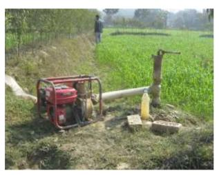
Figure 5 Diesel powered water pump near trial plot
