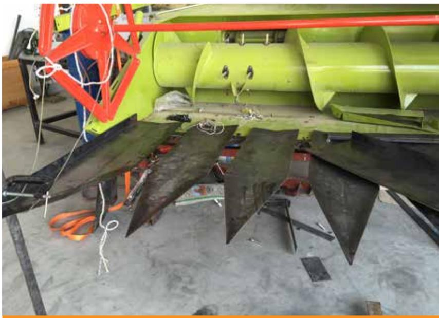
**Figure 26.** Sunflower trays fitted to the harvesting machine will reduce harvest losses. Photo: R. Martin.
