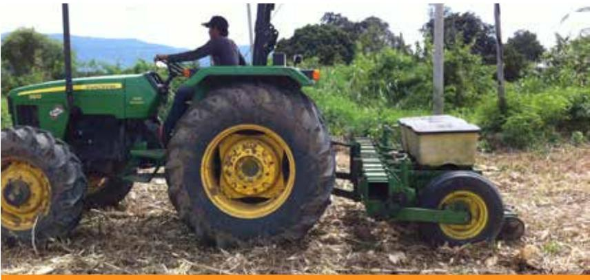
**Figure 5.** No-till planting into 5 t/ha maize residue using a three-row John Deere Maxemerge planter. Photo: R. Martin.
