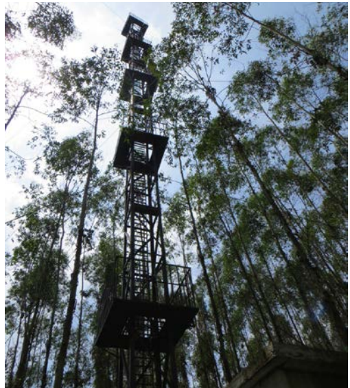
Figure 7. Instruments for measuring net water and carbon flux are mounted on this tower at Qipo Forest Farm near Nanning, Guangxi Province, China.
