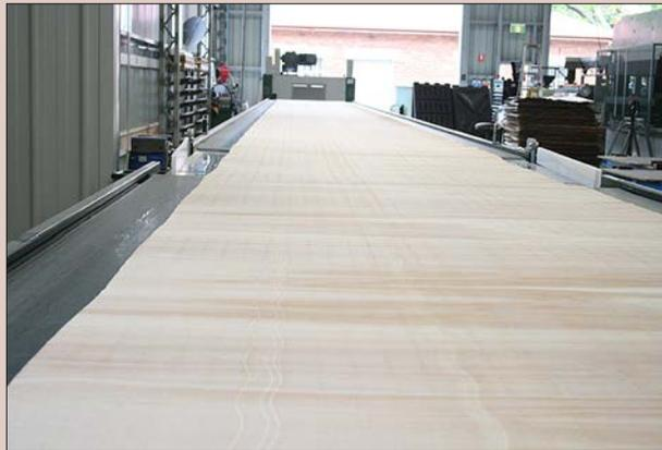
between the lathe and clipper. Using this information, unacceptable defects (e.g. large knots) can be limited to narrow strips of veneer that can be clipped out and rejected. The remaining veneer ribbon is clipped to sheet widths that best suit the final end product. This approach maximises the recovery of veneer with acceptable qualities, operates at speeds that equal the lathe operating speeds, and also produces more accurately sized veneer sheets.
