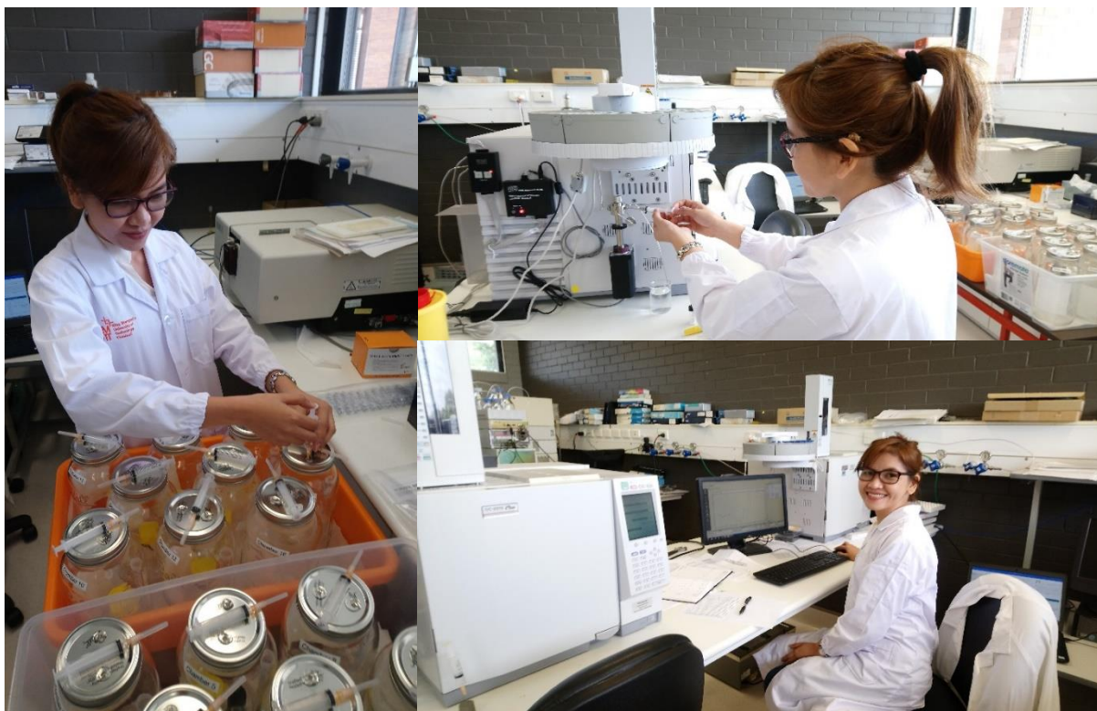
10-14 December 2018— Sampling of ethylene and measuring it with a gas chromatograph during a collaborative research on release kinetics and maximum ethylene release in Ripestuff™ conducted in UQ Gatton with Dr. Melinda Perkins.
