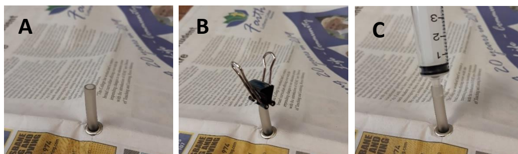
Figure 4. Headspace sampling of baskets was achieved via (A) a 5 cm length of 4 mm i.d. silicone tube fitted to a 5 mm i.d. eyelet in the newspaper lining. A metal clip was (B) used to pinch the tube closed during the experiment and (C) temporarily removed to facilitate sample collection with a 5 mL syringe.
