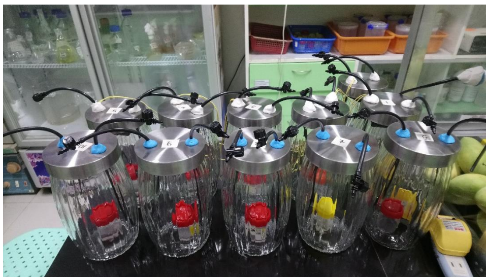
Figure 34. Glass jars with or without fan containing Ripestuff™ in a vessel with different number of holes (0, 1, 2, 3, or 4) in the lid.
