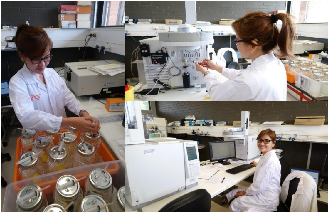
Figure 5. UPMIn team member Angelyn Lacap undertaking headspace sampling (left), sample injection into a gas chromatograph (top right), and subsequent quantification of ethylene (bottom right) during her visit to UQ in December 2018.
