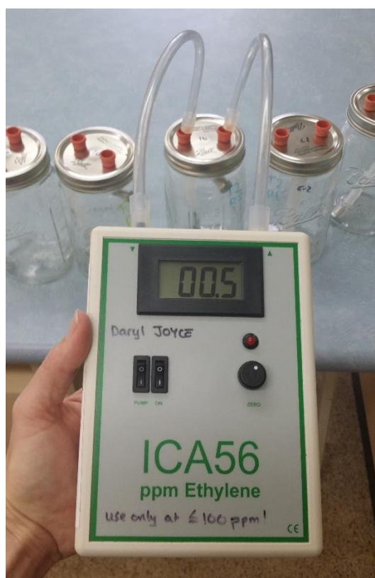
Figure 5: Image showing the ICA-56 ethylene sensor device measuring concentrations ( \mu L L^{-1} ) from silicone tubing inside the 1 L glass chamber via Suba-seal ® bungs and PVC tubing.
