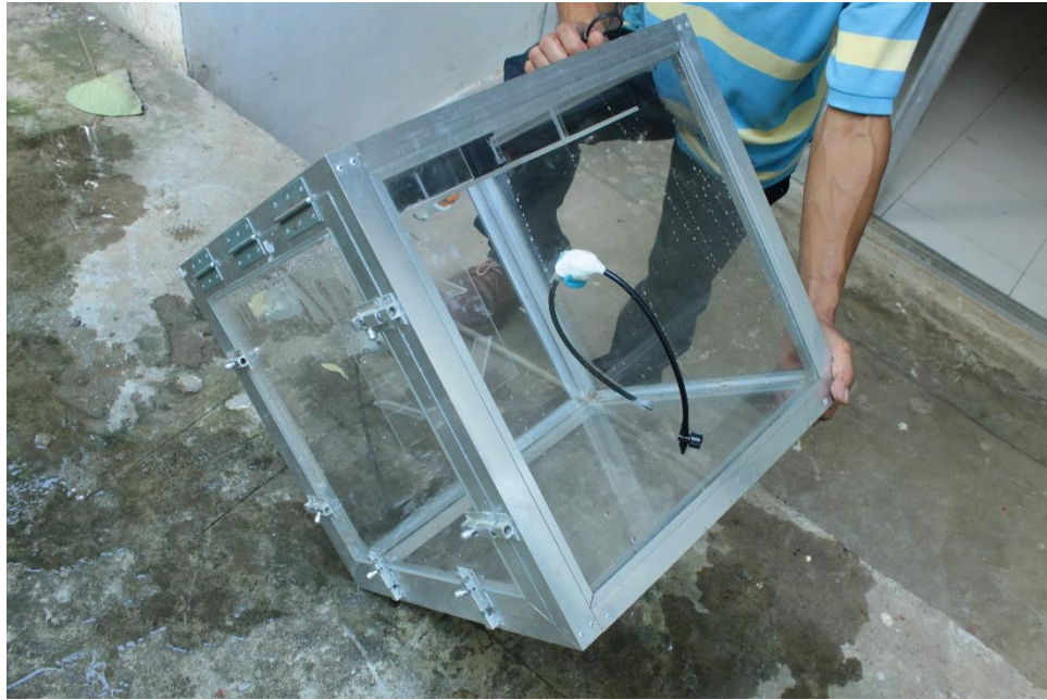
Figure 27. Leakage detection in chambers using water leak test.
