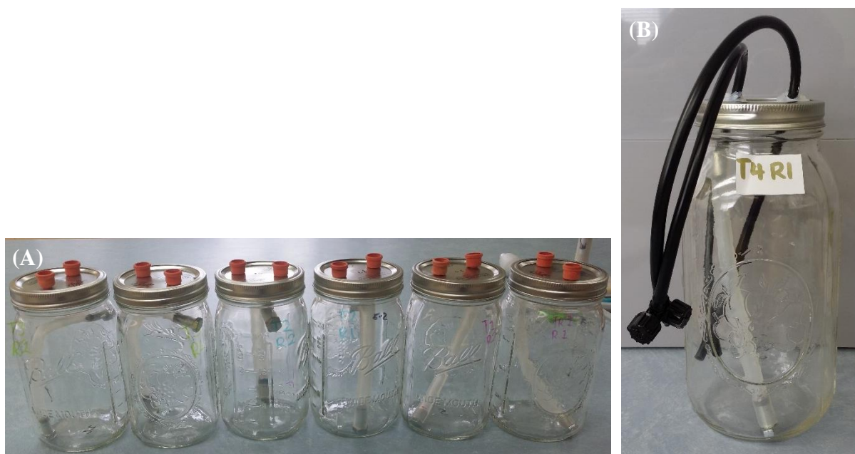
Figure 3: One (1) L chamber system with Suba-seal ® serrated bungs in lids (A) and 2 L chamber system with in- and out-flow tubes with micro taps attached to permit gas sampling (B).
