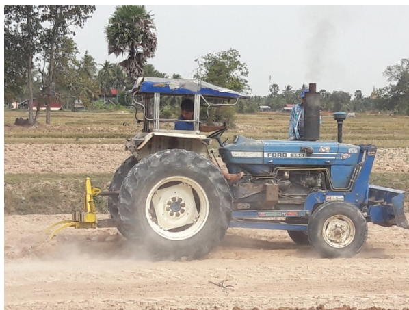
Photo 5. Deep ripper in action
