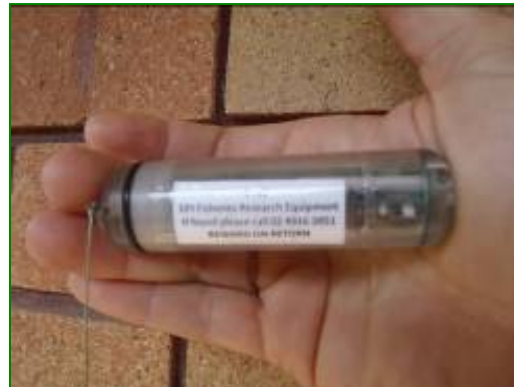
Autonomous sensor (Sensorfish) used to determine hydraulic conditions during weir passage
