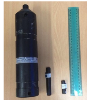
An acoustic receiver and two transmitters of different sizes. The smaller transmitter is the type used in the Black Bass Project.
