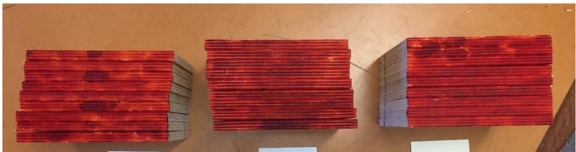
Figure 23: FR treated plywood with chemical test indicating retardant penetration.
