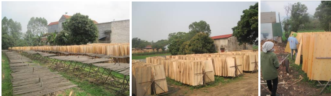
Figure 6.8. Examples of uncontrolled veneer air-drying at the surveyed mills
