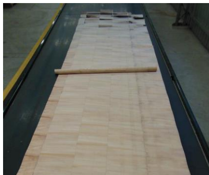
Figure 6.17. Knot-free hoop pine veneer (a) and veneer after drying (b)
