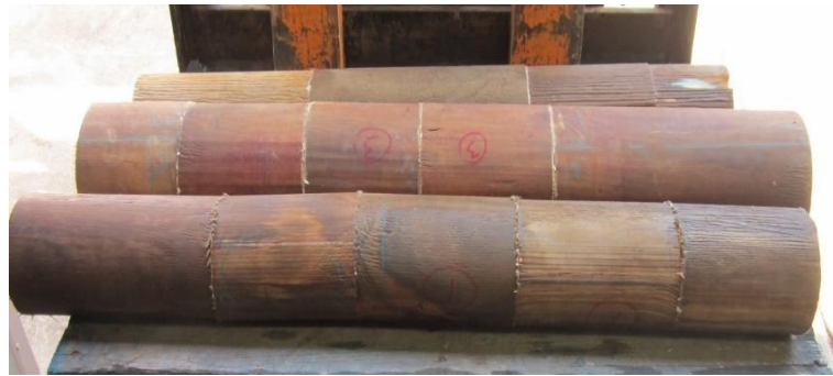
Figure 6.16. Pressed and glued green billets ready for peeling
