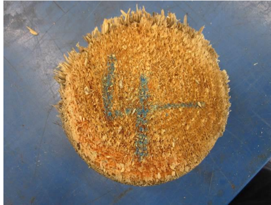
Figure 6.15. Surface roughening after cross-cutting with a circular saw
