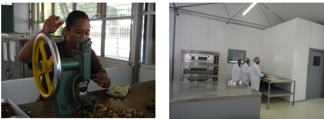
Figure 23. a) Cracking canarium nuts in the pilot factory. b) Inside the galip factory at the “clean” stage of processing
