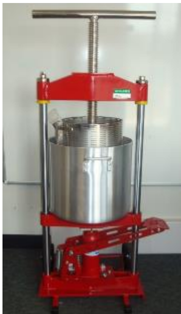
Figure 9. Coconut oil press from Axis Industrial Ltd (New Zealand) holds 15 litres meal per pressing.
