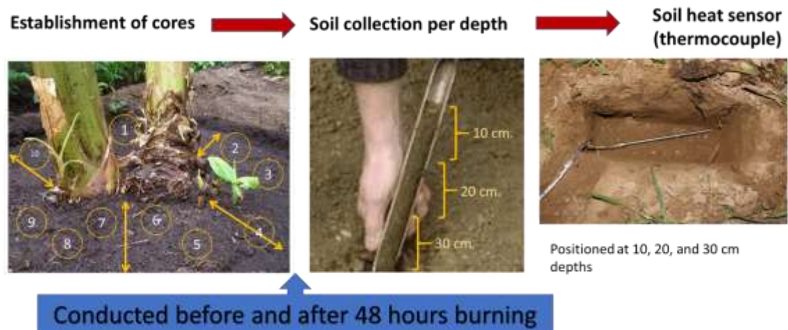
Fig 5.3. Diagram depicting the location of soil cores within the 30 cm band around the base of the infected banana plant before, soil samples collected at 0-10 cm, 10-20cm, and 20-30cm depth and placement of thermocouples.
