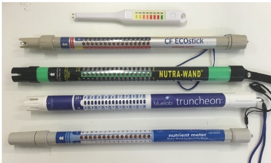
Photo 2: Five hydroponics salinity meters sourced from an internet search; top to bottom: HomeMed Salinity Checker, CF ECOSTick, Green Nutra-Wand, Blulab Truncheon and Nutrient Meter
