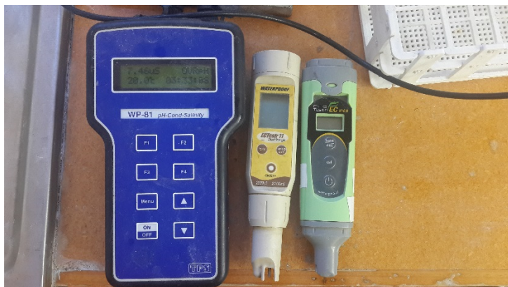
Photo 7. Three EC measuring devices used in the experiment; 1) TPS WP-81pH-cond-Salinity 2) ECTestr11 and 3) ecoTestr EC High
