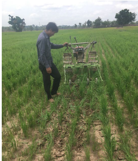
Figure 2: The unsuccessful attempt at inter-row cultivation with a tined implement in relatively dry soil conditions.
