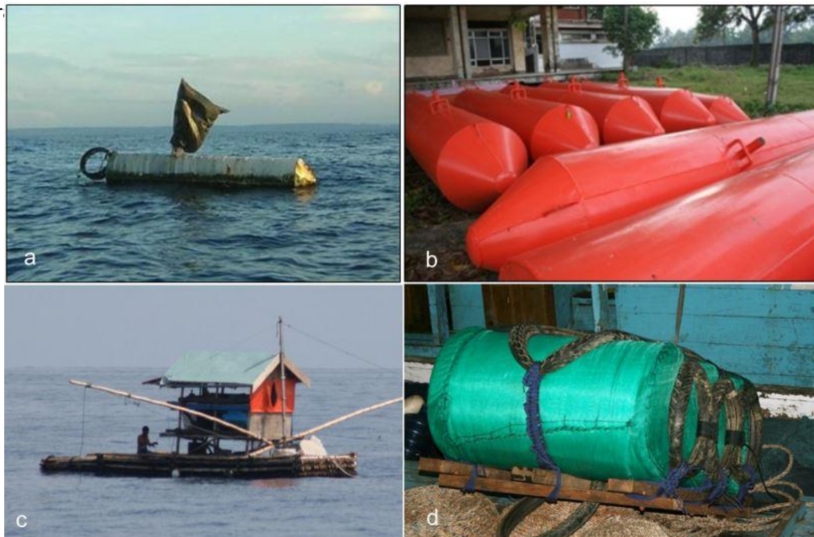
Figure 5.2. Types of anchored FAD floats in Indonesia (a) & (b) steel ponton , (c) bamboo raft with rakit , and (d) polystyrene gabus (photos: C. Proctor).
