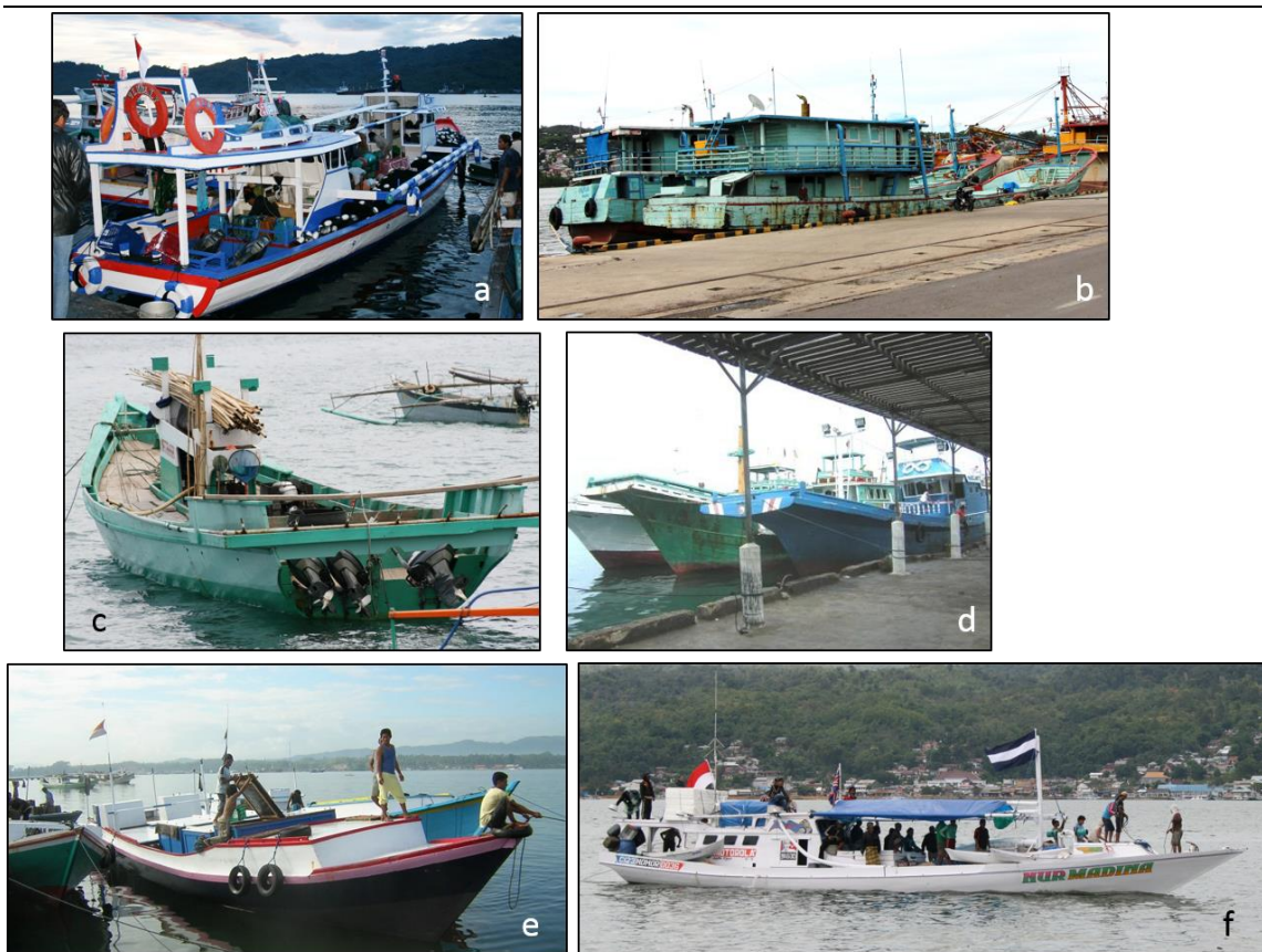
Figure 5.4. Examples of Indonesian vessel types that fish on FADs: (a) Mini purse-seine ( pajeko ), < 30 GT, at PPP Sodohoa; (b) larger purse-seine ( pukat cincin ), > 30 GT, at PPS Kendari; (c) small pole and line ( funae ) in Belang, North Sulawesi; (d) pole and line, >50 GT, in Sorong; (e) hand-line/troll-line ( penongkol ) at PPP Sodohoa; and (f) hand-line/troll-line 'mother-ship' carrying several small catcher boats ( sampan ) in Kendari (Photos: C. Proctor). From: Widodo et al. (2016).
