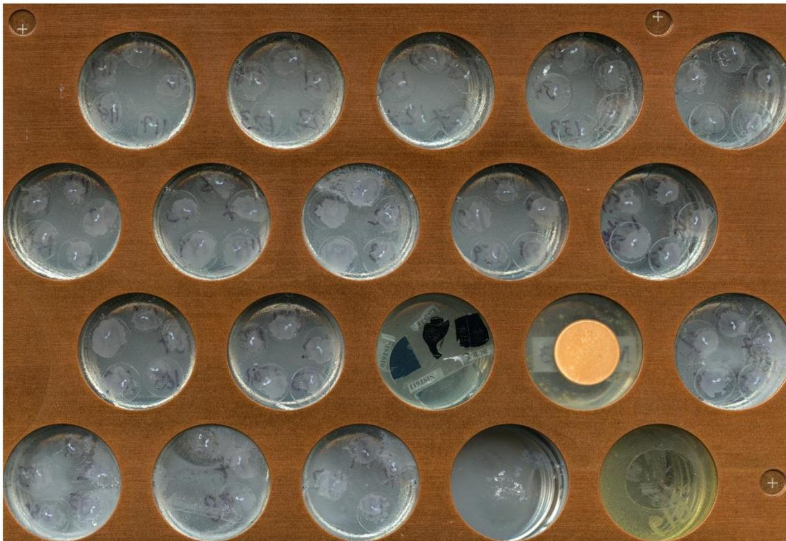
Figure 6.16. A holder with sixteen 1-inch rounds, each holding 5 otolith sections. The remaining positions in the holder contain reference standards.
