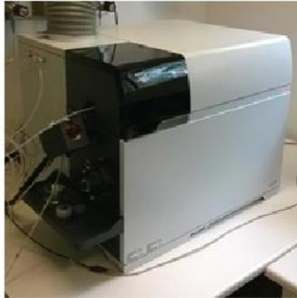
Quadrupole ICP-MS instrument used in study.
