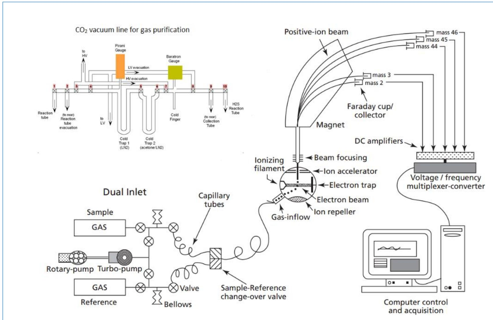
Figure 6.3. Setup of an isotope-ratio mass spectrometer measuring  $\text{CO}_2$ .
