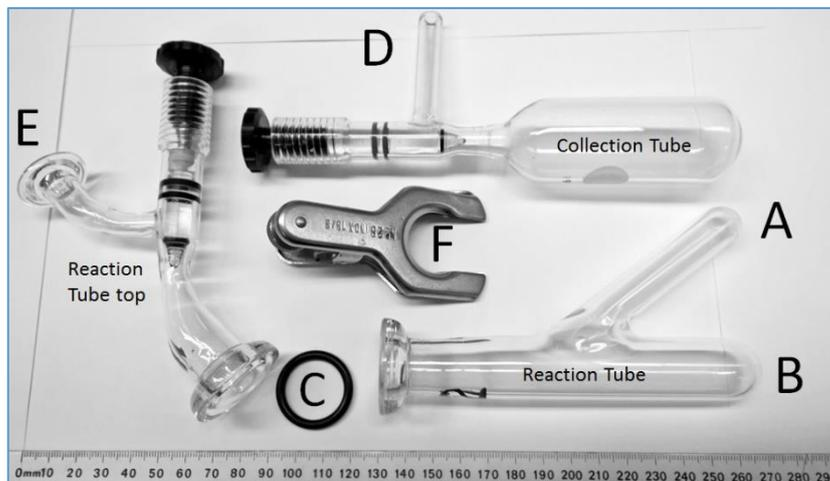
Figure 6.2. Glassware used for otolith digestion.
