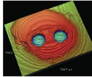
Optical profiler image of ablation crater in the mineral zircon. Crater formed after 12 seconds of ablation and is ~ 4 microns in depth by 29 microns in diameter.
